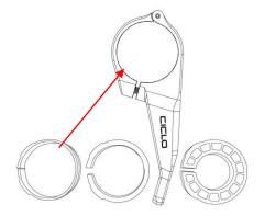
To mount the bracket to the bike you have to open the screw on the handlebar bracket. Then put one of the suitable rubber bands in the ring of the handlebar bracket, open it and put it at the desired mounting location to install the Handlebars.
