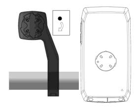
To fix the device in the holder, insert it to the left into the handlebar holder and turn it slightly to the right until it clicks into place. Please always check before cycling that the NAVIC 400 is correctly fastened.
